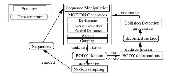
Figure 6. The system control flow of TRACK.
