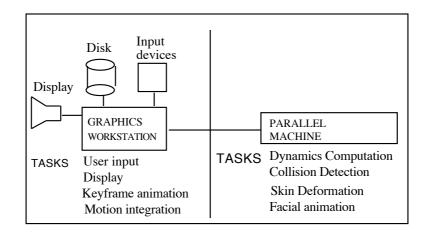
Figure 11. Architecture of the system.
